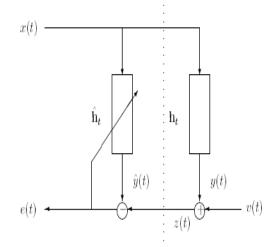
Fig. 1. Echo cancellation system. A. Performance of an Adaptive Algorithm
